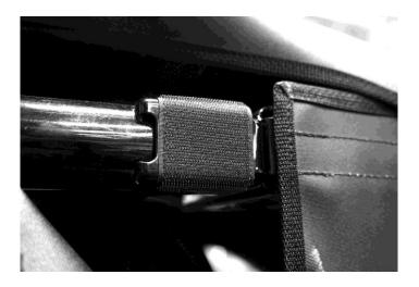
12. Then take the Rear Door and zip it to the Middle Rear Window. This ensures the door is properly placed. Then attach the top front corner to the Velcro. See photo below.
