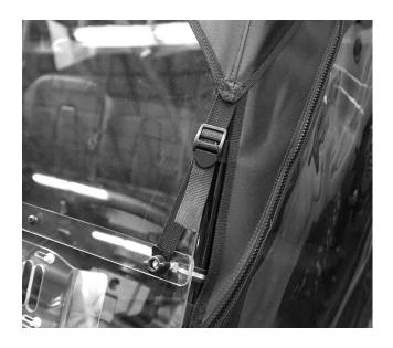
21. Next take the other two straps with Velcro sewn on one end and wrap them around the roll cage in the rear just under the Rear Door. Be sure to wrap the 6" adhesive strip completely around the bar and then tightly wrap the double-sided Velcro around the adhesive strip. See photo below.
