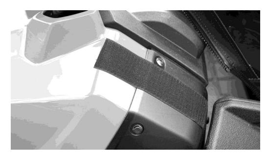
7. Last Item on the doors will be a snap on the inside front section of the plastic doors. It's easier to place the snap in the right position by first putting the screw snap stud into the socket on the enclosure. Then pull the door into place and push the snap into the plastic so that a mark is left. Then pull the snap out and screw it into the door making sure not to over tighten and strip out the plastic. See the photos on the next page.
