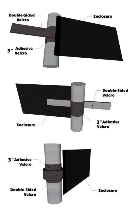
5. After attaching the double-sided strips go to the rear of the door. You will see three Velcro tabs sewn here. Starting just below the top cross bar place the 32" adhesive strips down the bar facing the rear of the vehicle. Then pull the tabs around and attach then down the bar to the Velcro. See photos on next page.
