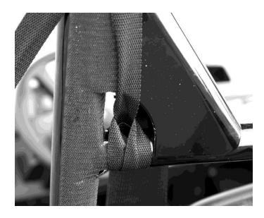
23. Now place the top over the entire vehicle, the front of the top is identified by the sides being more steeply curved, and begin by lacing the front straps through the ladder lock buckles sewn to the front corners of the top. Diagram below shows how to use ladder buckle.
