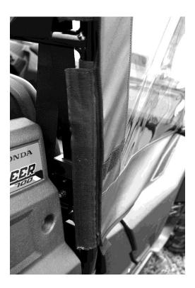
6. Now move to the front lower corner and place the 9" adhesive strip to match up with the Velcro on the cab. See Photo Below.
