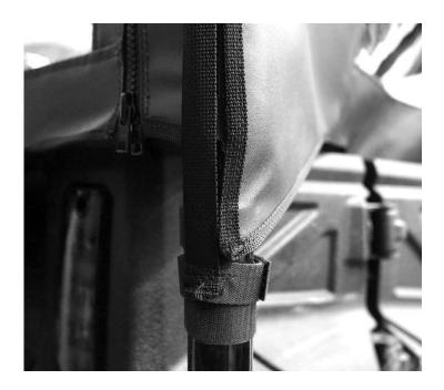
22. Next take the middle straps with loop sewn on one end and wrap them around the roll cage on the cross bar. See photo below.
