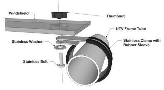
6. The middle Slot is where the two pieces overlap. Connect this the same as the other two except use the 1 1/4" bolt instead of the 1". See photo below.
