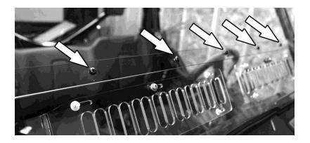
5. It's time to install the windshield on the vehicle. There are three slots on either side; the top slot gets a 1 7/8" clamp and the bottom two get 1 3/4" clamps. Start with the bottom and top slots using 1" bolts, washers, and a thumb nut as shown in the diagram below.
