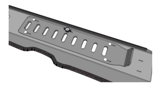
4. Now install the lower portion to the upper portion using the nylon bolts. There are five holes in both section with the holes in the upper portion being bigger. Set the upper portion on top of the lower portion and screw them together making sure that the slots on the ends are lined up. The photo below shows how this looks.
