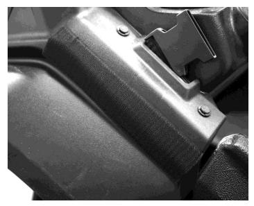
2. Next hold the door up to the frame and attach these spots then continue attaching it using the double-sided Velcro strips sewn perpendicular to the edge of the door. At each of the double-sided strips take one of the 3" adhesive Velcro strips and adhere it to the inside of the frame. Then wrap the double-sided strip around it so that the adhesive strip holds it firmly in place. The following diagrams show how it should look.
