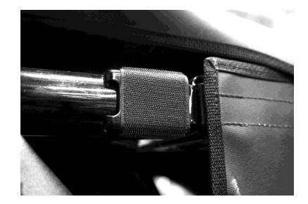
2. Then take the Rear Door and zip it to the Middle Rear Window. This ensures the door is properly placed. Then attach the top front corner to the Velcro. See photo below.
