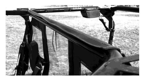
6. Next attach the double-sided Velcro strips down the side bars. Start at the top and work your way down the tube. See photo below.
