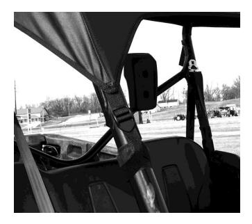
4. Next take the other two straps with Velcro sewn on one end and wrap them around the roll cage in the rear about 10-12" below the Top Cap. Be sure to wrap the 6" adhesive strip completely around the bar and then tightly wrap the double-sided Velcro around the adhesive strip. See the following photo.
