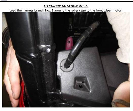
Connect the harness branch with the wiper motor connector.
