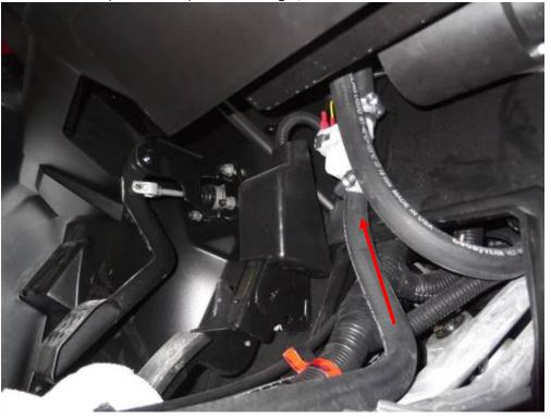
Install the short hose and remain of the hose to the heater tubes. Fix these hoses with the heater tubes by tightening straps and tighten these straps very hard. Insert the tightening strap onto the shorter hose and install electromagnetic valve in same orientation like in picture. Tighten that strap very hard.
