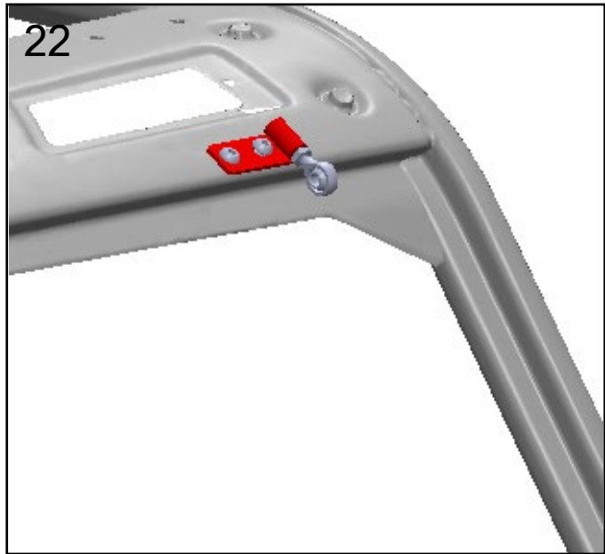
Use a 5mm hex and a 13mm socket wrench to loosely fasten two M8x16mm button head bolts and two M8 Nylon Lock Nuts for each Hinge Half, Upper on each side of the vehicle. Driver side shown
