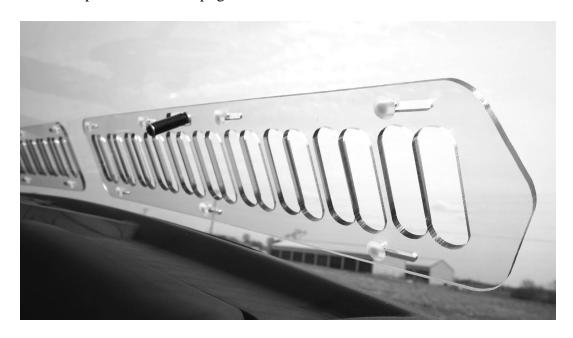
6. Now place the windshield inside the frame of the U-Force. Make sure that the windshield is set down into the space between the dash and the hood. Take the Metal brackets and bolt them to the windshield from the inside using the supplied 1" bolts washer and thumbnut as shown in the picture below.
