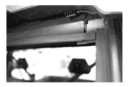
4. Next take the two vent slider and install then to the inside surface of the windshield. Start by installing the handle first. Take the 2"bolt, black spacer and lock nut and install them into the round holes on the sliders. Make sure that the bolts are installed on opposite sides of the sliders so that you have mirror images of each other when done. The pictures below show how to install the bolts.
