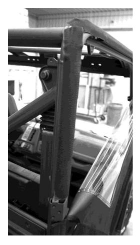
7. Next place the 5" strip just below the bracket along the back of the roll cage
