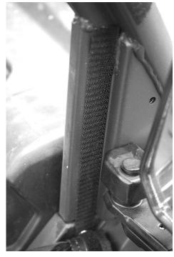
9. Lastly install the snap studs into the plastic for the bottom portion of the door. It works best to put the screw studs into the snap sockets on the door first. Then one by one pull the door in place and push the screw into the plastic
