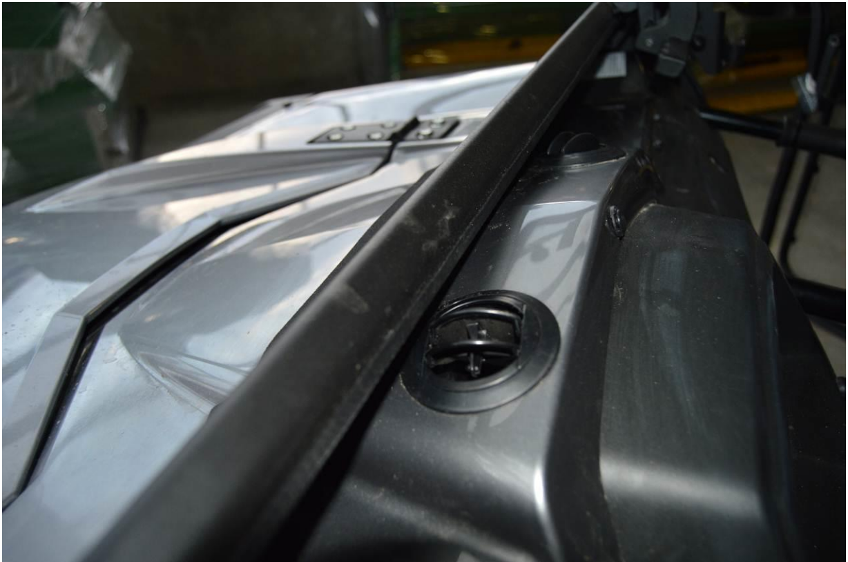
Cut 2 Ø50mm holes into the middle part of upper dashboard cover into the best position.
