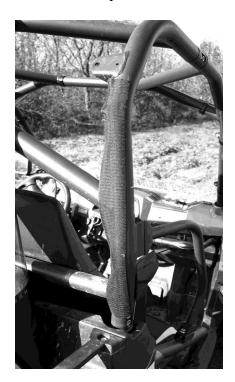
3. Once all the Velcro is in place the last thing to do is install the screw snap studs. NOTE: The best way to install the snap studs is to put them in the sockets in the door first. Then push them into the plastic to make an mark. Then pull the screw stud out and screw it into the plastic where the mark was made. See Photos Below.
