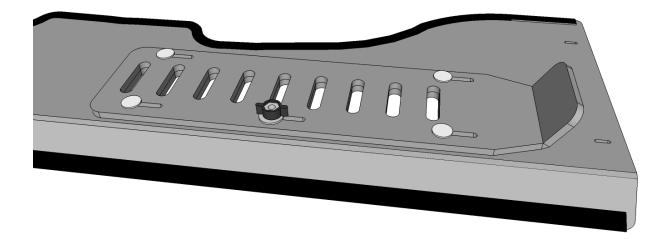
4. Now place the windshield inside the frame of the Defender. Take the Metal brackets and bolt them to the windshield from the inside using the supplied 11/4" bolts washer and thumbnut as shown in the picture below.
