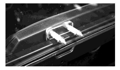
9. Once the Rear Window is in place and properly centered on the vehicle the final step is to install the brackets across the top of the window to secure it in place. This is done the same as the bottom brackets except you use no spacer. See photo below
