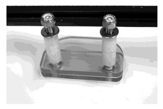
8. Now that the gasket and bottom brackets are in place it's time to place the Rear Window in place on the vehicle. The brackets are designed to hold the window in place along the bottom of the frame in behind the seats as shown in the photo on the next page.
