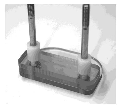
6. Now take the two plates and spacers and insert them into the holes along the bottom so that the plates are on the inside or the gasket side of the windshield. See photo below.
