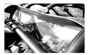
4. The sides of the Rear Panel will attach to the Downward bars on the inside facing the front of the vehicle. See the photo on the next page.
