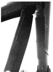
5. Lastly the middle of the window will attach to the center bar using the 40" adhesive Velcro
