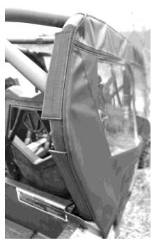
5. Next take the 10" and 4" adhesive Velcro strips and place it on the around the door in several locations as shown in the photo below. Then affix the bottom of the front panel to it as shown in the second
