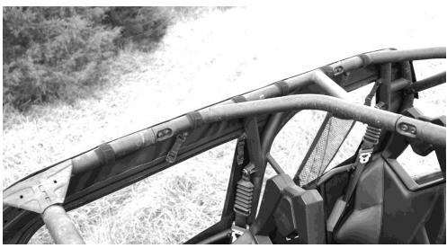
4. Next take the 30" adhesive Velcro strip and run it down the back of the roll cage facing towards the rear of the vehicle. They should match up with the double-sided Velcro tabs sewn along the rear of the soft door. See photo below.
