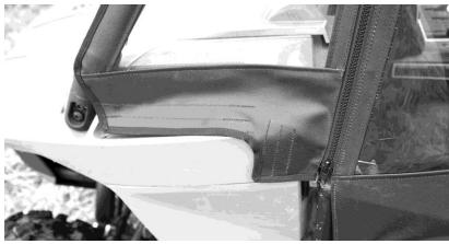
7. Lastly, attach one last double-sided strip at the bottom rear of the front door as shown in the photo below.
