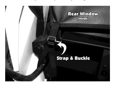
6. Apply the 6" and 12" adhesive Velcro strips between the horizontal bars facing the rear of the vehicle. Then attach the sides like you did the previous points along the top of the Rear Window. The photo below shows how this will look once done.
