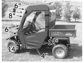
5. At the top of the front area and toward the bottom, you will notice strips of double sided Velcro. You will use the provided 6" adhesive hook strips with these. Below are photos showing how to attach these.
