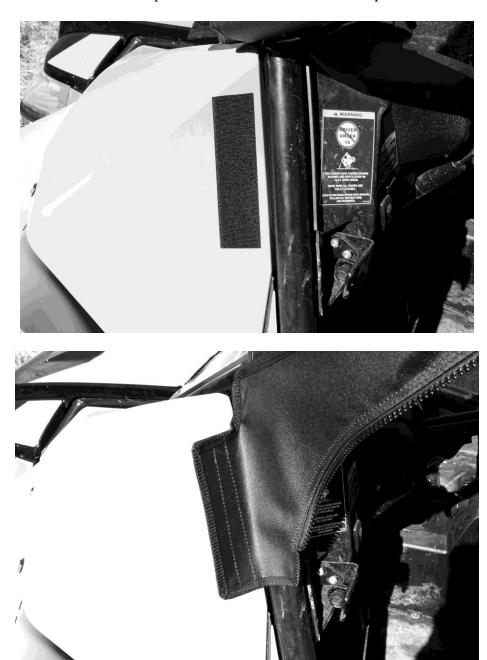
4. Last part of the door to attach is the bottom to the factory half-door. Take the 44" adhesive Velcro strip and attach it to the factory door to match up with the Velcro sewn to the bottom of the soft doors. The adhesive Velcro will cross the hinge of the door, take a knife and cut the adhesive Velcro at the hinge.
