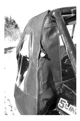
7. The bottom will attach to the vehicle using the 40" adhesive Velcro strip on the inside of the cab behind the seats as shown in the photo on the next page.
