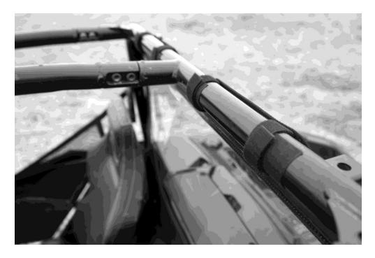
6. Next attach the sides of the Rear Window to the Velcro down the sides from the back of the Rear Window as shown in the photo below.
