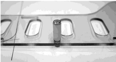
5. Now insert the bolt in the small holes and screw on the lock nuts so the end of the bolt is flush with the outside edge of the lock nut. Make sure that you place the bolt through hole on each slider so that they are mirror images of each other.
