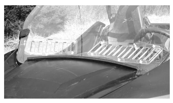
3. Next prepare the vent slider to be installed on the windshield. Take the two hex head bolts, 4 nylon spacers and two lock nuts and attach them to the vent sliders as shown in the photos on the next page.
