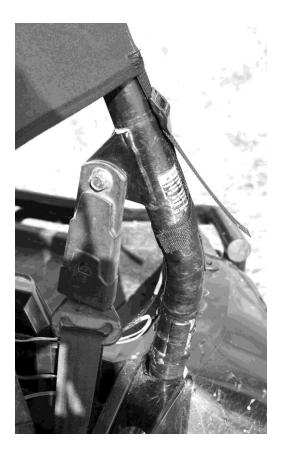
3. Once all the straps are in place run them through the buckles. Pull them tight making sure the top is centered and the side seams line up correctly along the roll cage. The diagram below shows how to lace the webbing through the buckle.
