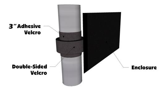
2. Next take the 10" and a 3" adhesive Velcro strips and run it down the back of the roll cage facing towards the rear of the vehicle. They should match up with the double-sided Velcro tabs sewn along the rear of the soft door. See photo below.
