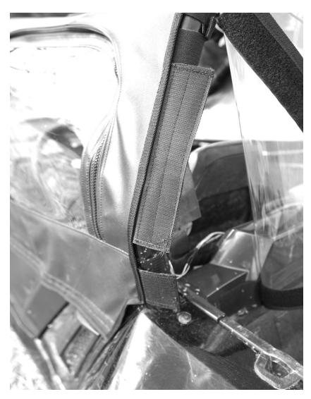
3. Next take the 6" adhesive Velcro strip and place it on the front fender as shown in the photo below. Then affix the bottom of the front panel to it as shown in the second photo.
