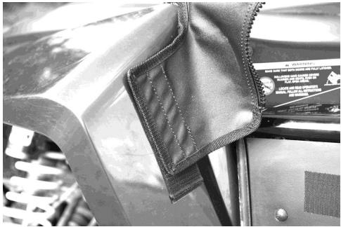
4. Last part of the door to attach is the bottom to the factory half-door. Take the 44" adhesive Velcro strip and attach it to the factory door to match up with the Velcro sewn to the bottom of the soft doors. The adhesive Velcro will cross the hinge of the door, take a knife and cut the adhesive Velcro at the hinge. See the photos on the next page.
