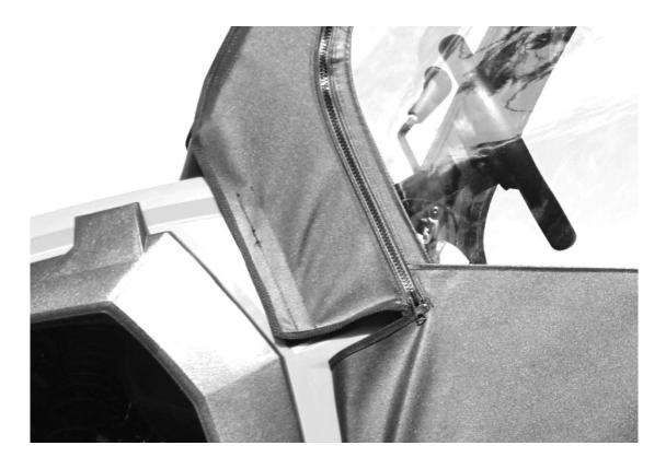
10. Now take the 18" Strip that is 1" wide and place it on the inside front portion of the factory door. Then take the bottom front section of the soft door and wrap it around the factory door and attach the two together as shown in the photos below.
