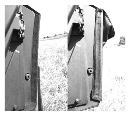
11. Lastly install the snap studs into the plastic for the bottom rear portion of thee door. It works best to put the screw studs into the snap sockets on the door first. Then one by one pull the door in place and push the screw into the plastic making sure to put enough pressure to leave a mark. Then remove the screw stud from the door and install it where the mark was left behind at. The following picture show what it looks like.
