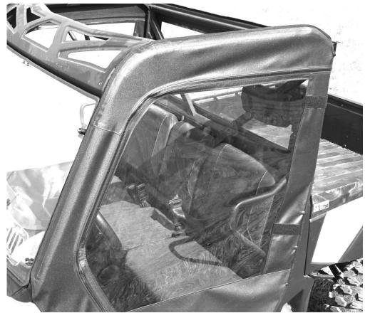
8. Next attach the 8" adhesive Velcro strip to the bottom of the front top portion of the door as shown in the photos below.
