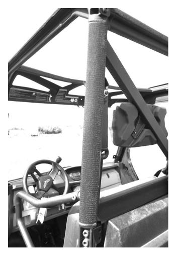
7. After all the Velcro is in place take the door and place it on the vehicle. The following series of photos show how it should look after being installed.
