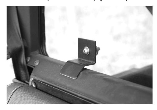
4. Next place the Rear window on the frame of the Prowler and hook the brackets on the bottom of the frame as shown in the photo below. You will need to get someone else to hold the Rear Window in place in order install the remaining brackets.
