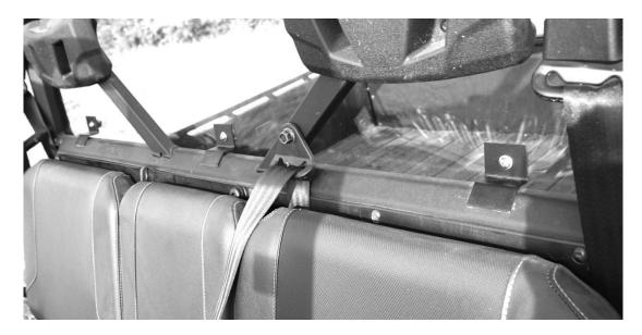
5. Now install the rest of the large brackets across the top and down the sides of the Rear Window. They are made to grab hold of the frame and pull the window tightly against the frame as shown in the photos below.
