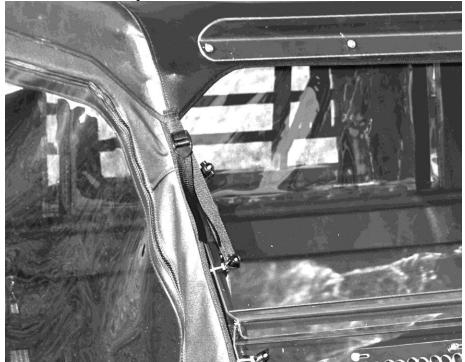
The rear of the Top Cap is held in place using the straps that have double-sided Velcro sewn in one end. Take the 6" adhesive Velcro strips and wrap them around the roll cage approximately 12" below the back of the Top Cap. Now take the end of the strap with the Velcro and wrap it around the bar and Velcro as tight as possible. Then take the other end of the strap and run it through the loop, pulling it tight. The photo below shows what it should look like.
