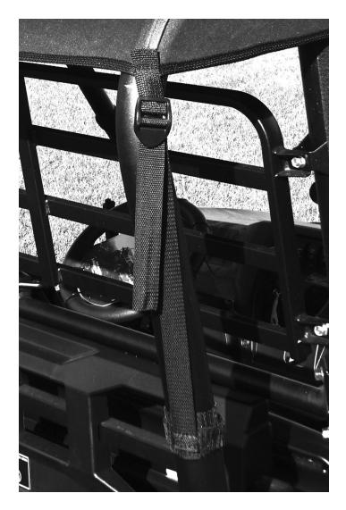
Once all the straps are in place run them through the buckles. Pull them tight making sure the top is centered and the side seams line up correctly along the roll cage. The diagram below shows how to lace the webbing through the buckle.
