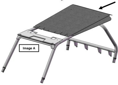
2. Make sure that the roof slides in under the OEM front visor and on top of the front crossbar so that the front edge of the roof closes the front visor opening areas and slots as shown on image B & C. Having a second person sitting in the vehicle to guide the roof into location is very helpful to achieve correct roof installation.
