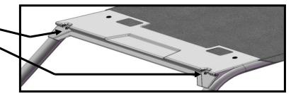
4. Finally, tighten the 2 rear mounting screws M6 x 40 to the roll cage.
