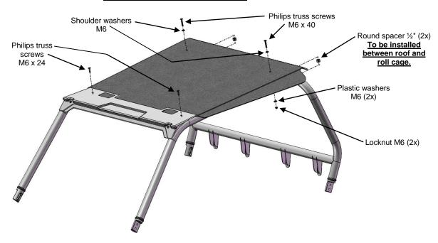
2. MAKE SURE that roof is PROPERLY positioned with the front visor (as shown in step d) and start tightening ONLY the front upper mounting screws M6 x 24 (2x) as shown below. This will make sure that the fit between the roof and the front visor will not move when tightening following mounting point.
