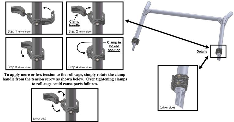
c) Install windshield to the clamps using supplied screws and washers without applying final torque. Ensure that the windshield and all clamps are properly positioned. Secure all clamps in locking position [Ref: Step 4 - section b] and tighten all screws as shown below.
