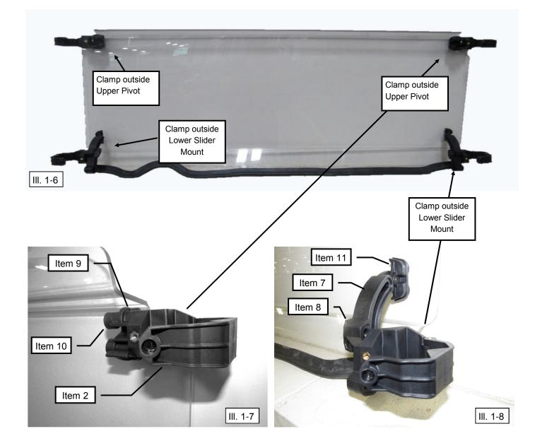
Ensure the clamps are open. With one person on the drivers side and one person on the passengers side, lift and position the Windshield Assembly onto the ROPS with the Bulb Seal (Item 13) sealing on the dash. See Illustration 1-9.
