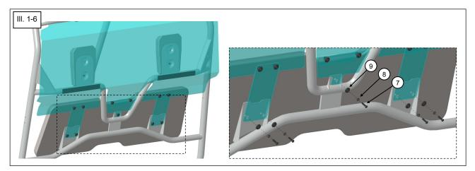
On both Headrests, position the Nylon Spacer [Item 11] between the Threaded Coupling Nut [Item 13] and the Upper Panel. Then insert the Domed Shoulder Washer [Item 9], Lock Washer [Item 8], and Button Head Screw - M6 x 26mm [Item 7]. See Illustration 1-7.
