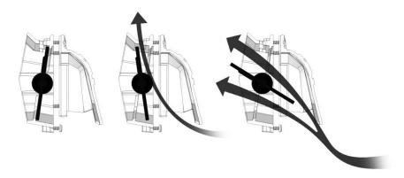
The vent has 3 positions: Closed, Defog, and open.
