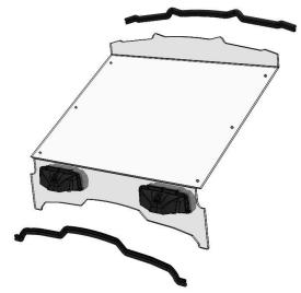
2. Push the 42" gasket on the top and the 46" gasket on the bottom of the windshield.
