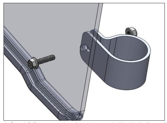
**2.** Snap 6 P Clamps onto the roll cage, 3 on each side with the flanges facing forward in the approximate locations of the mounting holes in the windshield. Mount windshield with the 6 bolts and nuts. Move windshield around as necessary for alignment before fully tightening.
