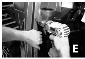
Step 6: Install new supplied U-Nut behind plastics of previously drilled hole. (See Figure F)
