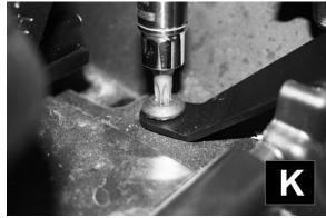
Step 12: Install hardware retained from Step 2 into upper two mounting holes on door hinge plate. Leave loose at this time. (See Figure L)
