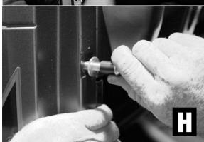
Step 9: Slide Drive side seat all of the way forward to access Torx head bolt located on the outside corner behind seat. For passenger side tilt seat forward to access same bolt. Set hardware aside it will be reused. (See Figure I)
