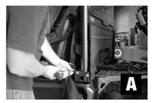
Step 3: Remove the two bolts and two pushpins from front "A" pillar step through. Two bolts and one pushpin will be reused. (See Figure B)
