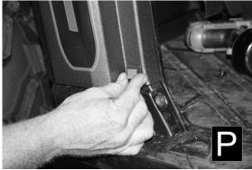
Step 17: Before tightening all hinge hardware, shut door to ensure that door frame aligns with plastics. Once preferred alignment has been reached tighten all hinge hardware. (See Figure Q)
