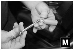
Step 14: Place supplied brass washers on the hinge mount pins. Apply anti-seize on hinge pins. Install door onto hinge pins and secure top hinge using supplied hinge screw. Thread locker is recommended to prevent screw from backing out.
