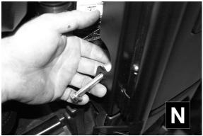
Step 15: Using a 4mm Allen wrench loosen 3 retaining bolts on latch and adjust to match alignment with striker pin. (See Figure O)
