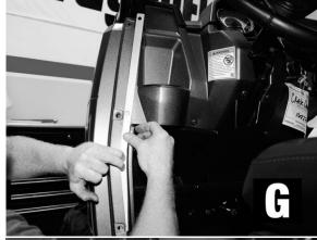
Step 8: Install supplied striker pin into 2<sup>nd</sup> hole down and thread into supplied U-Nut. At this time re-install previously removed factory hardware. (See Figure H)
