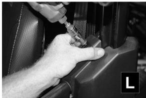
Step 13: Using supplied bolt, washers, and spacer. Place spacer and washer\*\* behind mid mount hole in hinge plate. Leave loose at this time. (See Figures M & N)
