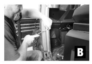
Step 4: Remove U-Nut located behind plastics in the second hole down location. Relocate this to the third hole down behind plastics. (See Figure C & D)
