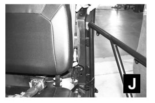
Step 11: Install hardware retained from Step 9 into lower corner mount of door hinge plate. Leave loose at this time. (See Figure K)
