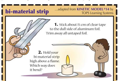
**3.** Aluminum and tape **expand** when heating, and **contract** when cooling.
