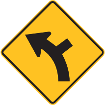
SIDE ROAD JUNCTION ON A CURVE
