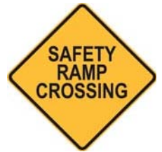
SAFETY RAMP CROSSING W5-31C W5-31D
