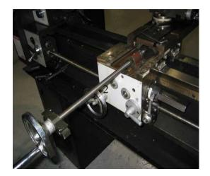
3. With the keyway facing down, the key will be Left inside the gear sleeve at the 6 o'clock position.
