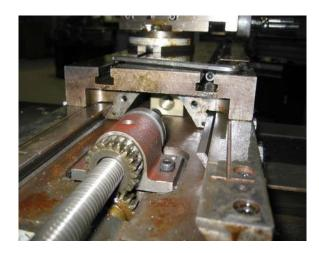
4. Remove the key (#22). Rotate the gear (#23) to the 12 o'clock position to make removal easier. Use a punch through the hole In the top of the Gear sleeve if necssary.
