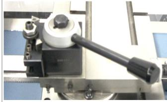
8 Holders can also be installed parallel to the machine bed as shown.
