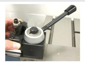
Use the knurled wheel to set the desired tool height with the workpiece. Then lock the hex nut down on top of the knurled wheel to lock it into place. This will allow the removal and installation of the tool and holder without the need to readjust tool height.
