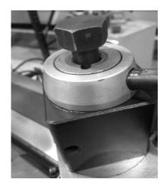
Rotate the handle counter clockwise and drop the selected tool holder and tool onto the QCTP.
