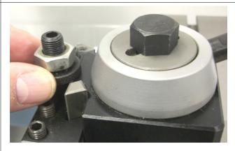
8 Rotate the handle clockwise to lock the holder into the QCTP.
