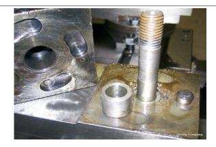
The last step in the installation is to place the QCTP over the stud and use the Chicago Bolt to secure it into place.
