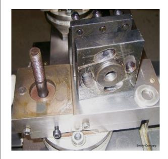
4 Later Granite machines have a stud with a removable sleeve. Lift the sleeve off the stud. It will not be used.
