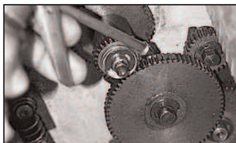
Figure 5.6 Oil the button behind the D gear.
