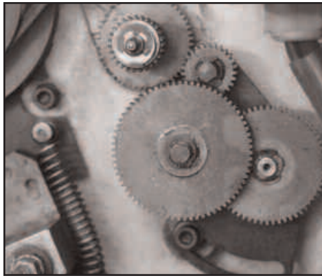
Figure 15.2 Slide the B and C gear shaft until the C gear meshes with the D gear
