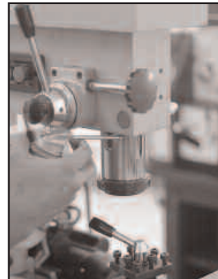
Figure 5.5 Oiling the Millhead Quill
