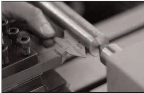
Figure 14.6 Use a center or thread gauge to correct cutter alignment error when squaring the cutter with the workpiece.
