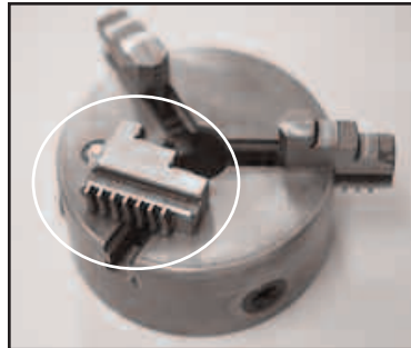
Figure 10.20 A serial number is stamped in the #1 slot of the three-jaw chuck.
