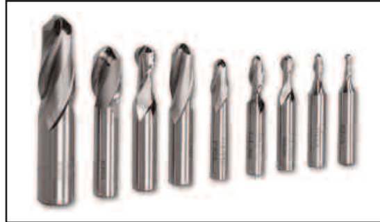
Figure 17.6 Ball end mills cut slots or fillets with a radius bottom
