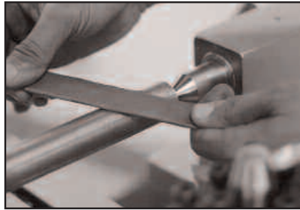
Figure 11.3 With a file, take full strokes at an oblique angle; never hold the file still.
