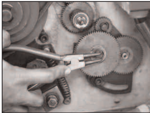
Figure 15.1 Remove all C clips, nuts, and gears
