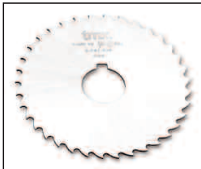
Figure 17.8 Side milling cutters are similar to plain milling cutter, but they have teeth on one or both sides
