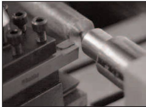
Figure 12.2 With a half-center you can extend the tool across the entire face of the work.
