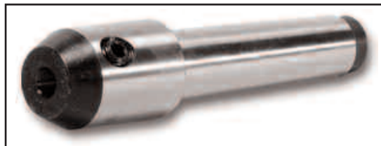
Figure 17.4 End mill holders also receive straight-shanked end mills.
