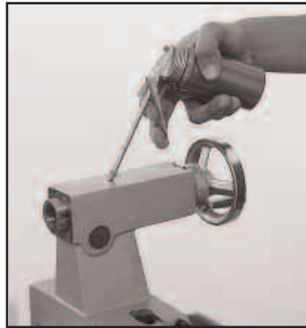
Figure 5.9 Oil the two buttons on the top of the tailstock.
