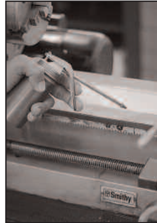
Figure 5.4 Oiling the ways
