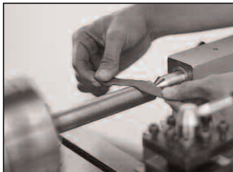
Figure 11.4 You can polish a workpiece with an abrasive cloth and oil.
