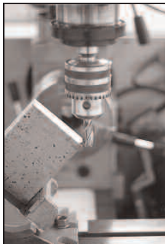
Figure 17.3 A bevel cut goes from side to side, completely removing the perpendicular edge.
