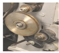
To set up for 24 threads per inch:
