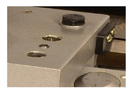
The quick change gearbox is oiled by removing the plug shown below and squirting oil into the opening. This oil will run over the gears inside the box and drip out the bottom of the quick change gear box. Oil in the drip pan below the box is normal. Oil daily or before each use.
