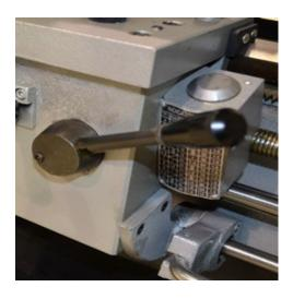
There is a reference mark on the threading dial housing and numbers on the dial. When the half nut is engaged the dial stops turning. By carefully engaging the half nut as the appropriate line or number passes by the indicator mark, a thread can be established and the lead maintained through the multiple passes that are required to cut a thread to the finished depth.
