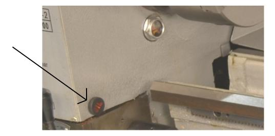
There are oil buttons located in numerous locations on the carriage, table, tool post and tail stock. These should be oiled on a daily basis. A 30 weight non-detergent oil is recommended.
