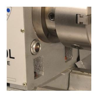
The apron has an oil reservoir. Oil is squirted one of the apron attach screw holes. It will run down into the apron. Oil should be half way up the site gauge on the front of the apron.
