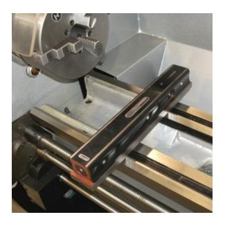
Move the level to the tailstock end of the machine. The bubble position should be the same as at the chuck end of the machine.
