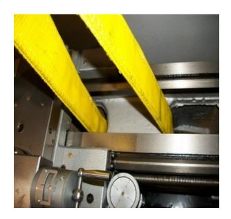
Attach the straps or chains to a hoist of forklift.
