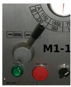
The Powerfeed engagement lever allows you to start the powerfeed for either the longitudinal direction or the cross feed direction. Moving this lever to the left and up will activate the power longitudinal feed. Moving the lever to the right and down will activate the power crossfeed.
