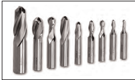
Figure 21.2 Ball end mills cut slots or fillets with a radius bottom.
