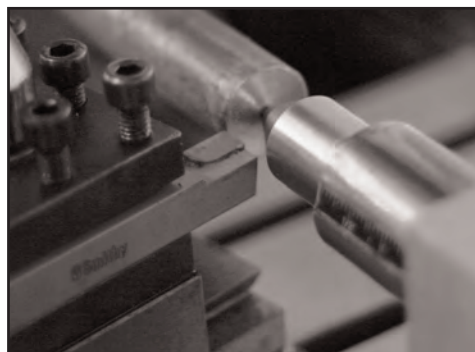
Figure 13.2 With a half-center you can extend the tool across the entire face of the work.
