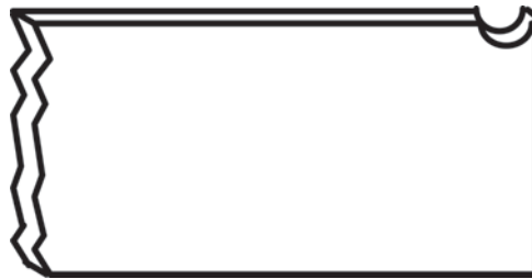
Figure 9.7 A crater starts the chip curling smoothly.
