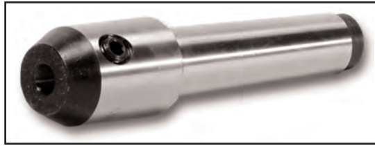
Figure 20.3 End mill holders also receive straight-shank end mills.
