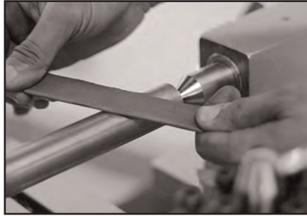
Figure 12.4 With a file, take full strokes at an oblique angle and never hold the file still.
