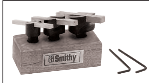
Figure 21.5 Flycutters take light face cuts from large surface areas.
