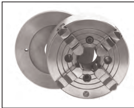
Figure 11.16 Four-jaw independent lathe chucks hold round, square, eccentric or odd shaped workpieces.
