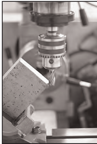
Figure 23.3 A bevel cut goes from side to side, completely removing the perpendicular edge.
