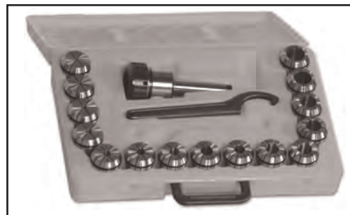
Figure 20.2 Spring collets, which fit into the mill spindle, hold straight-shank end mills.
