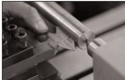
Figure 16.6 Use a center or thread gauge to correct cutter alignment error when squaring the cutter with the workpiece.
