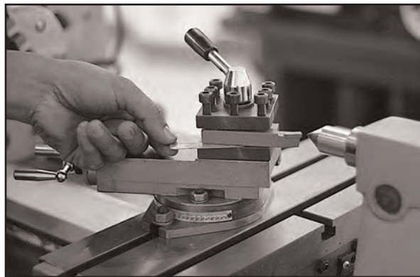
Figure 10.1 Placing shims under the tool can correct cutting too height.
