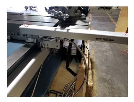
Before shipping Granite machines with factory installed DRO's, our technicians remove the Y axis scale and encoder to prevent shipping damage.
