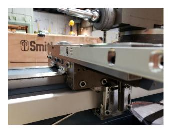
The holes for the mounting bracket have been predrilled and are located on the cross slide above the gib screws.
