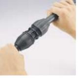
**2. PIPE INSERTION** Push pipe into the nut until the first point of resistance is met. There is no need to push the pipe in hard. Adequate pipe clearance is provided for all nut components.
