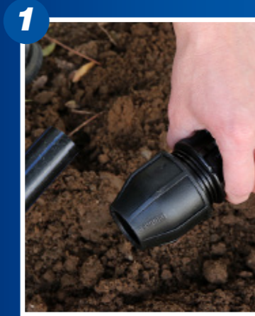
1 Cut the pipe square. There is no need to chamfer or lubricate the pipe. Ensure 3 threads are showing.
