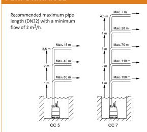
Installation depth: maximum of 10m below the water level.
