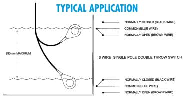
Switching range adjustable up to a maximum of 350mm depending on tethering point.
