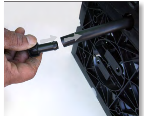
Insert the end plug of that row
