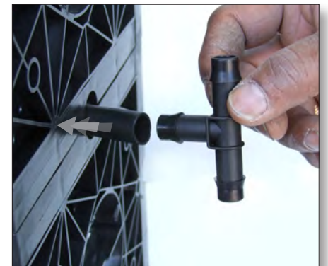
Insert the Tee-Connector at the other end
