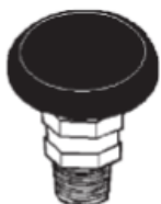
INSTALL VACUUM RELIEF IN COLD WATER INLET LINE AS REQUIRED BY LOCAL CODES.
