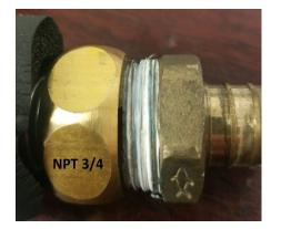
Bellows NPT ¾ to fitting connection
