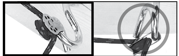
DIAGRAM 29. Align pigtail lag screws in direction of rope running through pulley.
