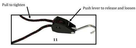
*The Bow & Stern tiedowns must connect to metal not plastic on the vehicle.*
