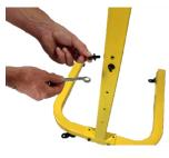
• Insert the *Post* with the black plastic cap into *Post* and secure with both sets of *Hex Bolts*, *Lock Washers* and *Washers*.
