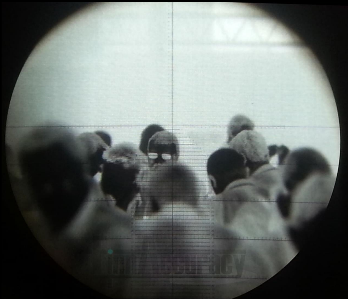
Competing milspec clip-on device with 640x480 resolution. Pixels clearly visible. Less thermal contrast on faces. Less depth of field, blurry background
